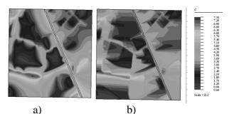
Figure 5. Dispersion calculation in cases of calm and the western wind.a) windless conditions; b) wind along an axis of abscissa of 3 m/s.
