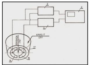
Fig.1.Amperometric and conductometric scheme of measurement principle with enzyme biosensor. 2acquisition electronics unit, data processing and display, 3-amperometric electronic unit, 4conductometric electronic unit, 10- silicone hose, 14,15-platinum electrodes, 17-cup, 21- pipette or manually electronic unit.
