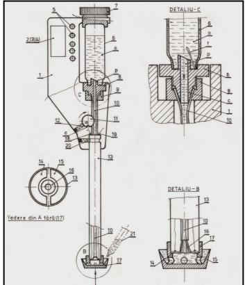
Fig.2.Sectional view of enzyme biosensors. 1-body 2- electronics unit of acquisition, data processing and display, 3-electronic amperometric unit, 4-conductometric electronic unit, 5-keyboard, 6- plastic capsule, o- oxidase solution, 7-bolt, 8-marker, p-drill, f-strip, c-con, 9-nut, 10-silicone hose, 11- supported eccentric cylinder l-conical seat, 12- ratchet, 13-bar 14.15-platinum electrodes, 16-con, 17-cup, 18.19- electric contacts, e-slot 20-ratchet ball, 21- pipette or manually hopper.
