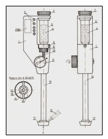
Fig.3.Exterior front and side of enzyme biosensors, 1-body, 2- electronic unit acquisition, data processing and display, 3-amperometric electronic unit, 4- conductometric electronic unit, 5-keyboard, 6- plastic capsules, o- oxidase solution, 7-bolt, 8-marker, p-drill, f-strip, c-con, 9-nut, 10-silicone hose, 11-cylinder eccentric supported, l-conical seat, 13-rod 14.15 platinum electrodes, 16-con, 17-cup, 21- pipette or manually hoppers.
