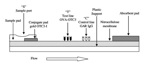
Figure 1. Schematic diagram of lateral-flow immunochromatographic assay
