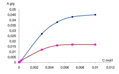
Fig.1 The adsorption is therm clinoptilolite modified by N, N-dimethyl-N-hexadecyl-N-2-oxyethlammonium bromide / rhombic symbol / and H-clinoptilolite / square symbol /
