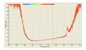
Figure 2. Graph chart recorded for a sample of nickel electrodeposited on copper substrate at -900 mV potential, temperature 65°C, time 2 minutes
