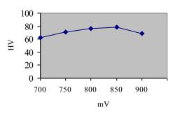
Figure 6. Micro-hardness vs. deposition potential
