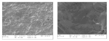
Figure 1. SEM images of the nickel electrodeposited layer from a Watts bath with addition of PVP at -700 mV potential, 65°C temperature, deposition time 10 minutes, with magnetic shaking of the electrolyte (SEM-Zeiss EVO 20 device)
