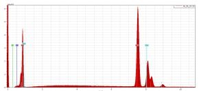
Figure 4. EDX pattern for a nickel sample electrodeposited on copper substrate at -750 mV and 60°C
