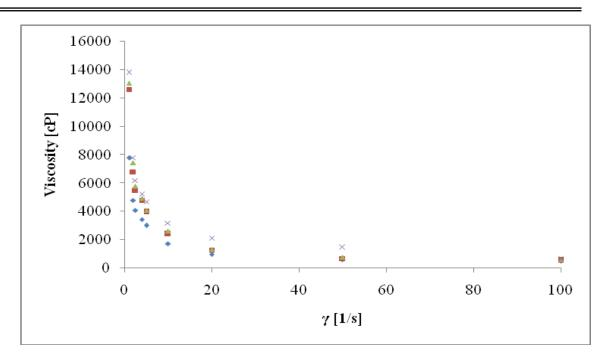
**Figure 1.** Viscosity profile of yogurt sample with corn flakes (cross - 1.5 g corn flakes, triangle - 2 g corn flakes, square - 2.5 g corn flakes, rhombus - 3 g corn flakes)
