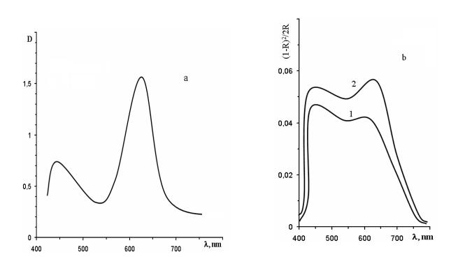
Figure 1. Absorption spectra: a – alcohol solution of the pigment; b – alcohol solution of the heterostructures P/TiO<sub>2</sub> (1) and F/P/TiO<sub>2</sub> (2)
