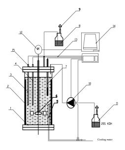
Figure 1. Scheme of the laboratory bioreactor 1 - vessel with geometric volume of 2 dm<sup>3</sup>; 2four repulse devises; 3-thermo-strength Pt100; 4-heater; 5-heat exchanger for cold water; 6turbine stirrer; 7-pH electrode; 8-exit for CO<sub>2</sub>; 9-filter; 10-peristaltic pump for pH correction; 11- reagent for pH correction - 20% KOH; 12motor; 13-control links; 14-control device "Applikon".
