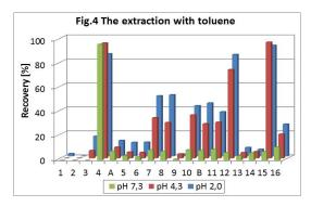
Figure 4. The extraction with toluene
