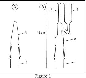
A: The glass extraction (volumetric) flask, equipped with a male joint (1) and conical stopper (5), prepared to microextraction. B: The solvent thin layer separator (2) containing side arm for water (3), capillary for extract (4) connected to the flask (1) after extraction.
