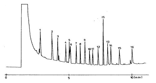
Figure 2. Chromatogram of model mixture of this chlorinated phenols (at concentration of each component of 10  $\mu$ g.l<sup>-1</sup> of water) in chloroform before extraction. For identification of peaks, see Table 1-3. IS = 1-Cl-n-octadecane.
