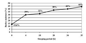
Figure 1. Steeping diagram for first experimental version
