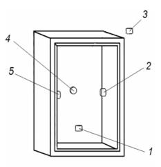
Figure 2. Location of the temperature probes
