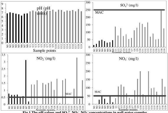
Fig.1 The pH values and  $SO_4^{2^\circ}$ ,  $NO_2^{-}$ ,  $NO_3^{-}$  concentrations in well water samples
