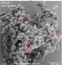
Figure 1. SEM image of the TiO<sub>2</sub> sample.
