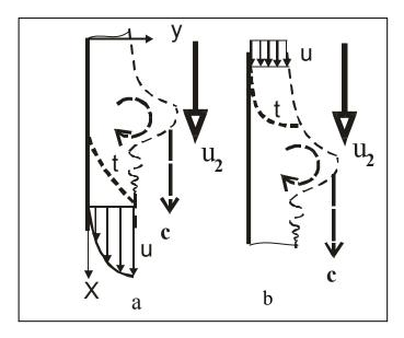
Figure 2. Schematic of big wave passage on the film surface a) velocity and temperature profiles prior to big wave passage; b) the same – afterwards
