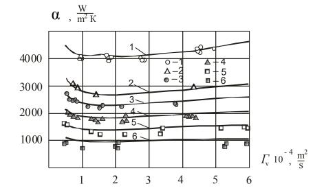
Figure 6. Comparison of experimental heat transfer coefficients (HTC) to water and sugar solutions free falling films with the calculated results by (34, 36) at λ<sub>bw</sub>=120 mm.
