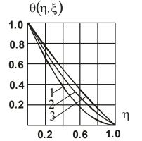
Figure 4. Temperature distribution in water film
