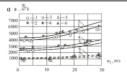
Figure 5. Effect of steam core velocity upon heat transfer coefficient. Water and sugar solutions at t = 100 °C. 1, 2 – water; 3, 4 – sugar solution, DM=40%; 5, 6 – sugar solution, DM = 70%.  $\lambda_{bw}$  =120 mm. Lines – calculated by (3, 34, 36, 37, 38)
