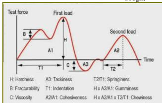
Fig. 1. Identification and quantification elements of primary and secondary parameters of texture profile analysis (TPA) performed in coordinates force - time [9]
