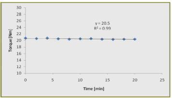
Fig.5. Variation in time of resistive moment of dough with 50% flour and 150 rpm of propeller stirrer.
