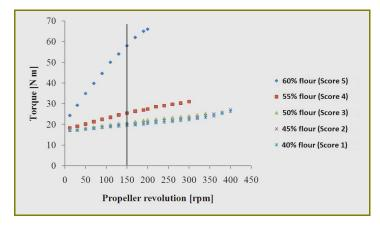
Fig.4. Graphic cumulative representation of resistive moment evolution depending on the speed at different concentrations of flour-water according to [1] and tab.2. highlighting resistive moment at 150 rpm
