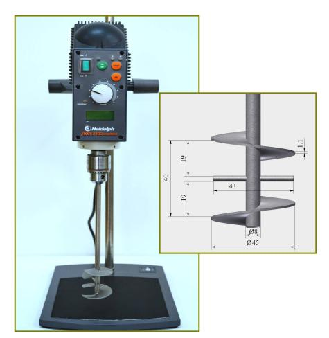
Fig.2. Schematic diagram of the experimental stand used for determining gumminess of semisolid food and view of the propeller used in experimental research.
