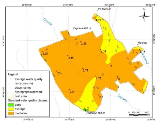
Fig. 8. The worst water quality classes (colour palette for: 1 – very good... 5 – deteriorated) and the arithmetic average (displayed numeric values on map) of all recorded water quality classes per each sampling point
