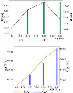
Figure 1. Farinograph characteristics of wheat flour-citrus fiber blends: ST, dough stability (min); DT, dough development time (min); SDg, softening degree of dough (BU); WA, water absorbtion (%).
