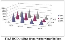
Fig.3 BOD<sub>5</sub> values from waste water before treatment
