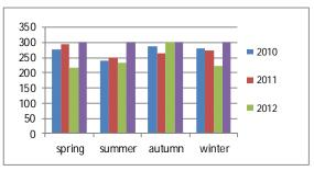
Fig.4. BOD<sub>5</sub> values in waste water after treatment
