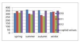
Fig.6 Values of suspended solids content in waste water after treatment
