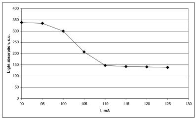
Figure 2. Dependence of the wanted signal value on the tube feeding current.
