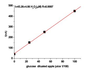
Figure 11. The glucose concentration determined in the tested samples
