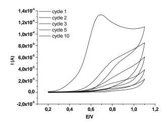
Figure 6. Cyclic voltammograms recorded during the formation of the monomer DHN – APEA on the SPCE / PB prepared via the galvanostatic method 10 mM APEA; 0.9 mM 2,6-DHN; 10 mV/s; 10 cycles
