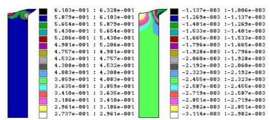
Figure 6. Allocation of a) movements and b) porosity in the bulk volume of dispersed material.
