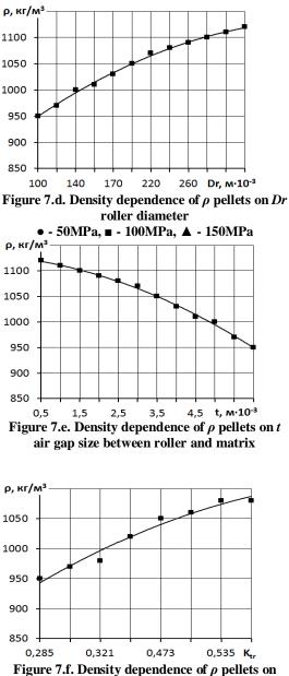
Figure 7.f. Density dependence of  $\rho$  pellets on friction coefficient between DM and matrix
