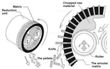
Figure 2. Granulator unit with annular matrix
