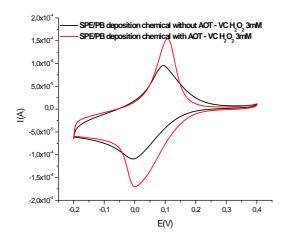
Figure 2. Cyclic voltamograms, in KCl 0.1 M in HCl 0.1 M; the scane rate 50 mV/s, modified PB/AOT using the chemical procedure.
