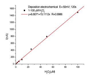
Figure 6. Calibration curves obtained by successive additions of solution  $H_2O_2$  phosphate buffer pH 6.5, E= -50 mV/s.
