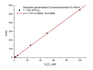
Figure 7. Calibration curves obtained for  $H_2O_2$  detection performed at electrodes with PB layers in the 1-100  $\mu$ M concentration range. Applied potential -50mV/s.
