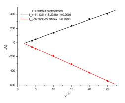
Figure 4. Variation of oxidation and reduction vs. square root of scan rate in electrolyte solution 0.1M KCl, 0.1M HCl
