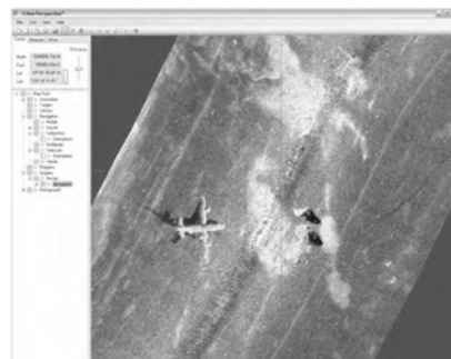
Fig.5. Image of plane wreckage obtained by post-processing of sonar signals (Source: ECA/ Triton Imaging Inc.)
