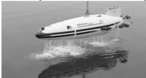
Fig.4. The Alistar-3000, inspection AUV - usable up to 3,000 m deep (Source: ECA)
