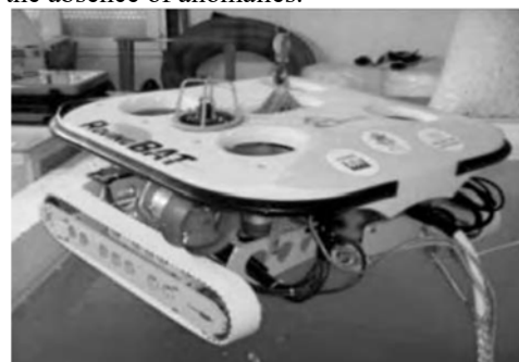
Fig.7. The ROV Roving Bat (Source: ECA)
