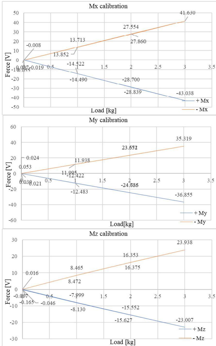
Figure 3 Calibration for the 6 components SMFM
