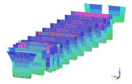
Fig.8 FSU 3D-FEM - transversal bulkheads
