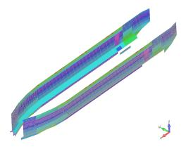
Fig.13 FSU 3D-FEM model – inner hull
