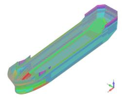
Fig.11 FSU 3D-FEM model – external shell
