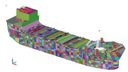
Fig.6 FSU 3D-FEM fully developed model
