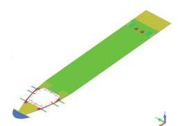
Fig.12 FSU 3D-FEM model – inner bottom
