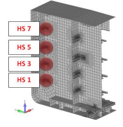
Fig.15 Structural details HS1,HS3,HS5,HS7
