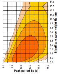
Fig.21 WNA wave scattering diagram [1].
