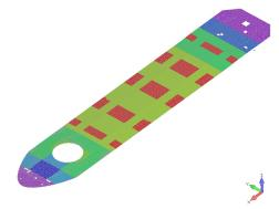
Fig.10 FSU 3D-FEM model – main deck
