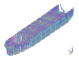
Fig.7 FSU 3D-FEM model – web frames
