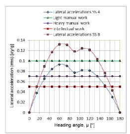
Fig. 19. Lateral accelerations for Sea States 4 and 8 compared to the acceptable limits for different activities.
