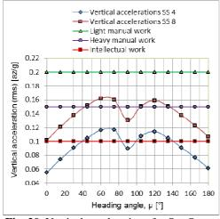
Fig. 20. Vertical accelerations for Sea States 4 and 8 compared to the acceptable limits for different activities.
