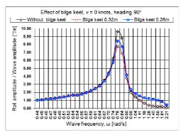
Fig. 17. Effect of bilge keel on roll motion attenuation, v = 0 kts
