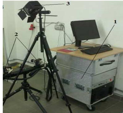
Fig. 7) Components of ARAMIS HS optical measurement system
