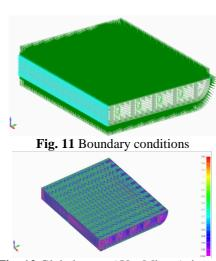
Fig. 12 Global stress (VonMisses), in case of the bordering lack
