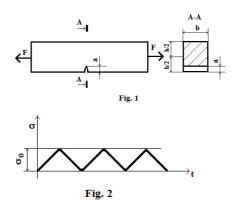
Fatigue or durability calculations are made by using Wöhler diagram, a diagram which is obtained experimentally through specific procedures applied for a long time. One should consider a rectangular specimen
