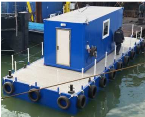
Fig.2. The floating container workshop in shipyard bay
