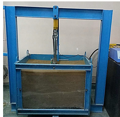
Fig. 4. Actual pile load test set-up with LVDT and load cell.
