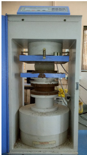
Fig. 2. Testing of mortar cube and cylinder in the CTM.
