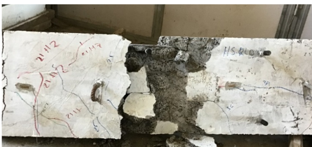
Fig. 15. Failure mode of the specimen HS-RL0.
