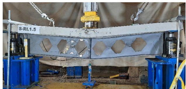
Fig. 12. Failure mode of the specimen S-RL1.5.
