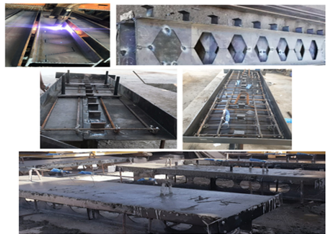
Fig. 1. Fabrication and cast of the composite castellated beams.
