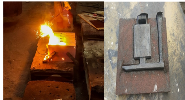
Fig. 3. The pouring moment-mold display after cooling.
