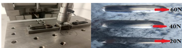
Fig. 6. Images of wear testing and specimen after wear test.
