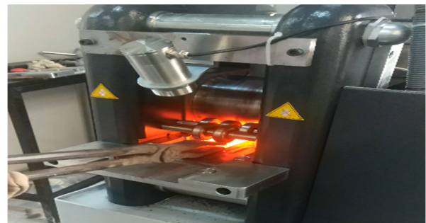
Fig. 4. Rolling process in laboratory conditions.
