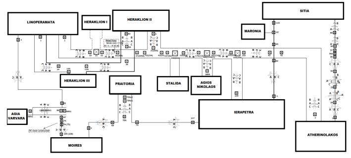
Fig. 2. Schematic of the Transmission System of Eastern Crete. Dotted lines depict undergound cables. Legal numbering of towers is given within parentheses when different from the operational numbering. Larger squares denote double circuit towers that support three circuits. Linoperamata and Atherinolakos are step up substations. The line connecting Heraklion II to the Linoperamata-Ierapetra line is referred to as System-Heraklion II.
