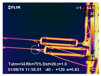
Fig. 16. A typical image acquired by a thermal camera from the ground showing a typical issue (a hot spot in the jumper connection).
