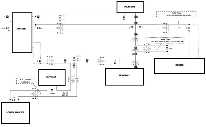
Fig. 3. Schematic of the Transmission System of Rhodes. Dotted lines depict undergound cables. South Rodes and Soroni are step-up substations.
