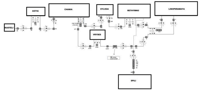
Fig. 1. Schematic of the Transmission System of Western Crete. Dotted lines depict undergound cables. Chania and Linoperamata are step-up substations. The Linoperamata-Rethymno-Eyligia-Chania line is referred to as Linoperamata-Chania I and the Linoperamata-Vryses-Chania line as Linoperamata-Chania II.
