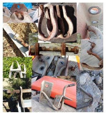
Fig. 7. A collection of pictures with various metal parts/fittings (shackles, clevises, bolts, pins, v-hangers etc) as removed from service.
