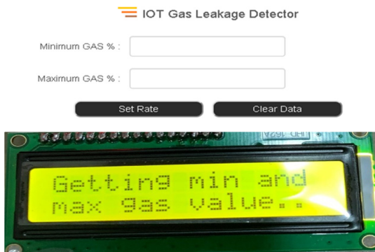
Fig. 9. Pipe minimum and maximum gas concentration values input when connecting to the server.
