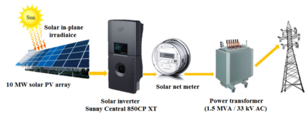
Fig. 1. Components of the grid-connected solar plant.
