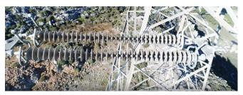
Fig. 4. The flashed under insulator with visible arc traces on rings. Sheath damage barely visible from this angle and distance.
