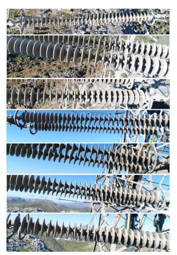
Fig. 10. Views of the flashed under insulator before its removal
