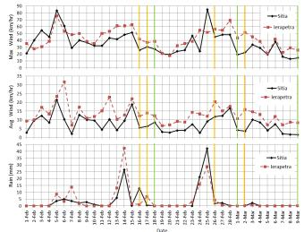
Fig. 11. Weather data from weather stations in the National Observatory of Athens network located in Sitia and Ierapetra. Yellow vertical lines indicate the occurrence of fault(s). Green lines indicate the re-energization of the line.
