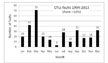
Fig. 12. Faults per month as recorded in Transmission Lines of Crete from 1994 to 2013.
