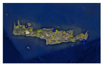
The Transmission System of Crete (screenshot from Google Earth. Fig. 2. Map data: Image LandSat/Copernicus) (yellow triangles: step-down substations, blue squares: step-up substations attached to power plants).
