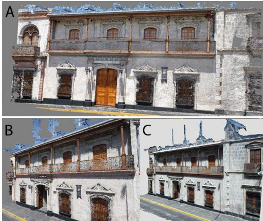
Figure 6. Results of point cloud format in photogrammetry (a) and aerophotogrammetry (b and c).
