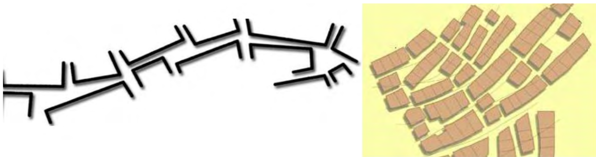
Figure 10. a (left): Depicts the street spaces and design that give more shade to pedestrians. b (right): Depicts the fabric of the village and provides Nubians with an experience similar to those of their original homes.
