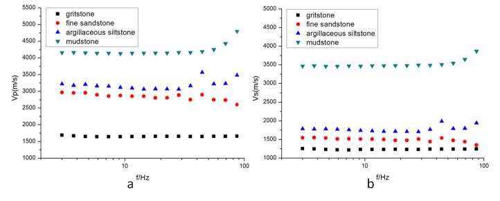
Figure 2. Relationships between the propagation velocity of sound waves in the four types of rocks and the frequency
