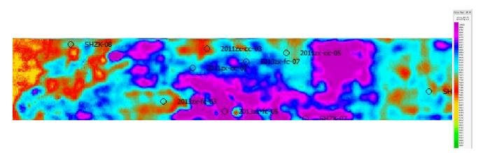
Figure 3. P-wave impedance properties of the #3 coal seam roof
