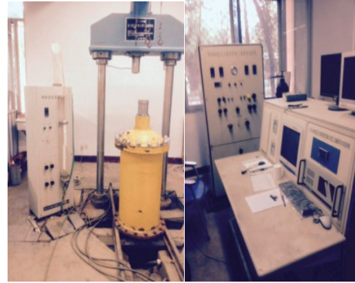
Figure 1. Large-scale triaxial apparatus of coarse-grained soil.
