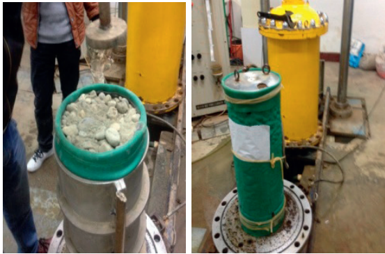
Figure 3. Large-scale triaxial specimen of sandy pebble soil.
