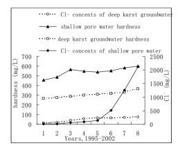
Figure 6. The Cl- contents and hardness of karst groundwater and shallow pore groundwater changing characteristic in the coal mining district.
