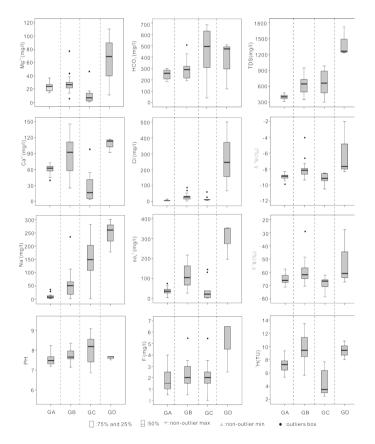
Figure 3. Box and whisker plots show the median of water quality parameters in the four clusters ( $GA \times GB \times GC \times GD$ ).
