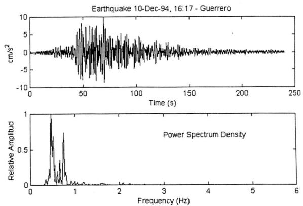
Figure 3. Signal in time (top) and frequency domain (bottom). Note the spectrum rarely exceed the 5Hz.
