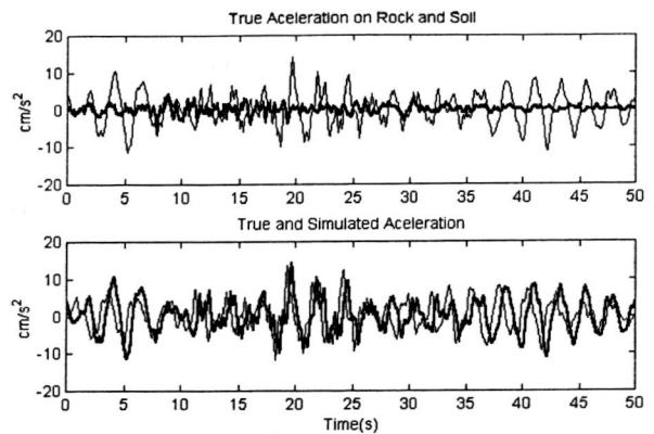
Figure 6. On the top, true acceleration on rock (heavy line) and (soft line) soil. On the bottom, true (soft line) and simulated (heavy line) acceleration for the same time window of soil.
