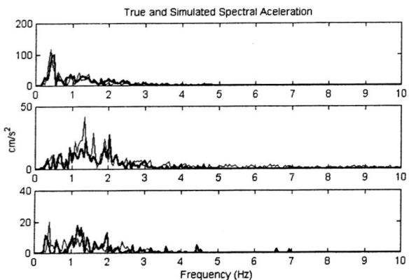
Figure 5. True (soft line) and simulated (heavy line) spectral acceleration on soil for three different records. The simulated data obtained from spectral acceleration on rock not taken in account in the training.
