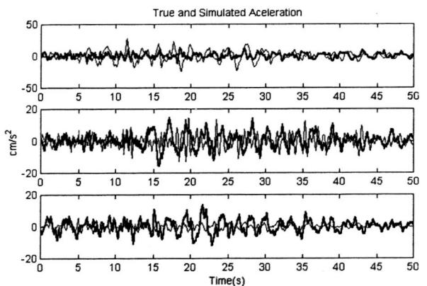
Figure 7. True (soft line) and simulated (heavy line) acceleration for three different events.
