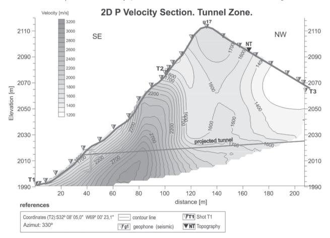
Figure 8. Seismic Refraction Tomography Profile.
