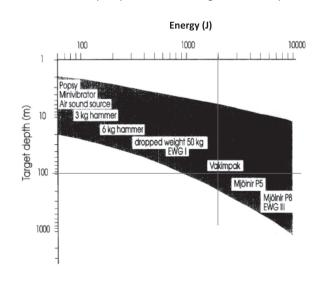
Figure 5. Amount of energy necessary related to depth of investigation for seismic sources (from Herbst et al, 1998).
