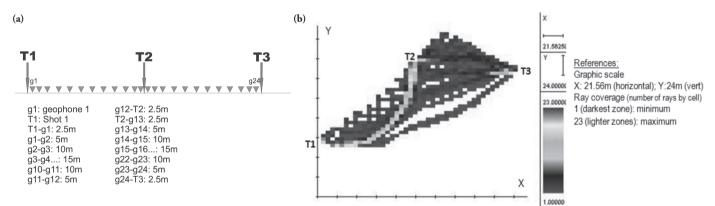
Figure 4. (a) 24 channels refraction seismic survey array and distances among stations. (b) Ray coverage for refraction tomography.
