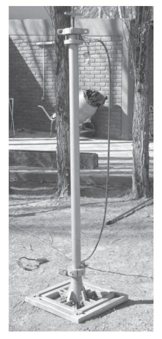
Figure 6. TAMPER. Vertical-Horizontal seismic wave generation system. Vertical implementation.
