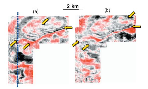
**Figure. 6.** Comparison of time slices on the full offset range for the: (a) conventional and (b) target oriented migrations. Slice is taken at 1.2 seconds, approximately the time of the target horizon. Faults trending to the NE can be identified between the yellow arrows in each image.
