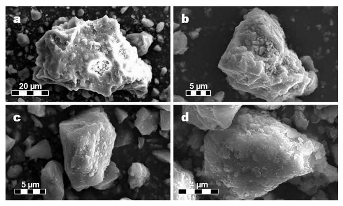
Figure 4. SEM images of natural clinker particles.
