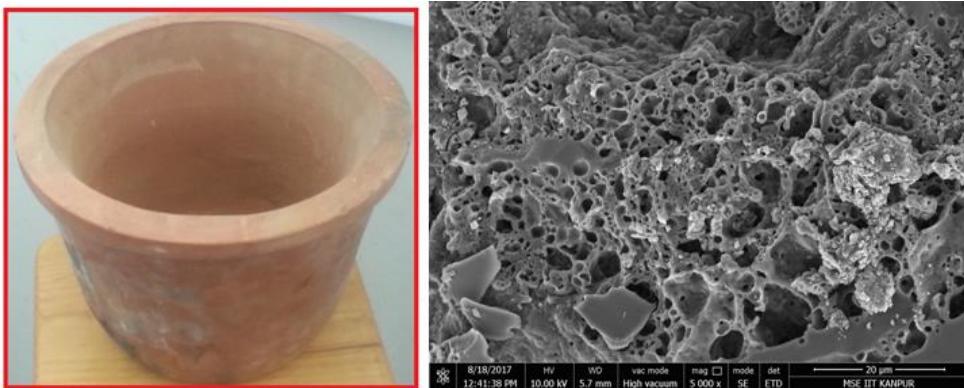
Figure 4b. SEM micrographs of the fractured surface of C60-25-15 sintered at 850°C.
