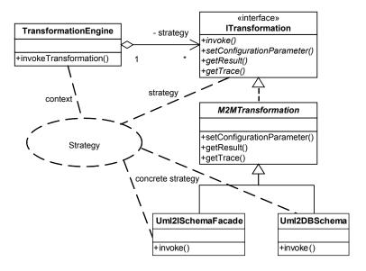
Figure 1: Architecture of the Transformation Framework
