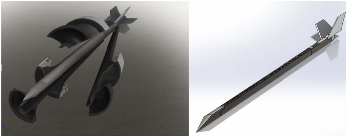
Figure 12. 3D model of APFSDS projectile 120 mm M829A2 [9]
