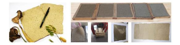
*Image 5: Paper. A laminate from a mixture of 80% water hyacinth fibre and 20% recycled newspaper, both previously treated with water immersion of 7 days to soften the fibre.*
